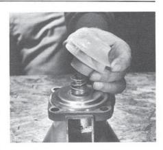
with metallic impellers, provide 96-144 in-lbs of torque.
